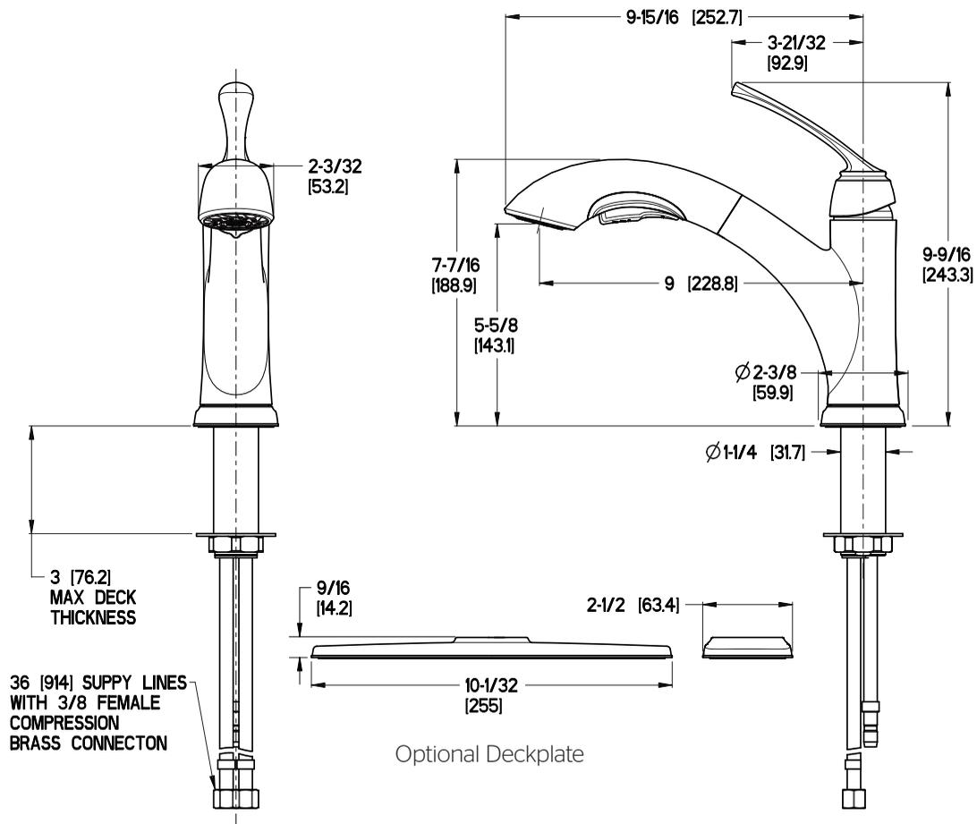
Ø1-3/8 Min to Ø1-1/2 Max. Deck Hole Openings
